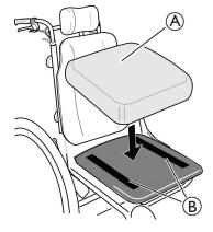
Depends of the cushion model, some seat cushion A can be secured with hook and loop straps B on the seat plate.
