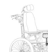
The height adjustment and removal is operated by the handwheel A.
